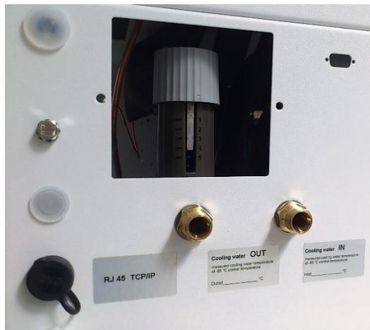
Fig. 2 Open cover of the cooling water volume regulator.
